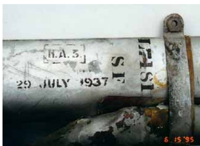
Identity revealed under clip on wing strut
